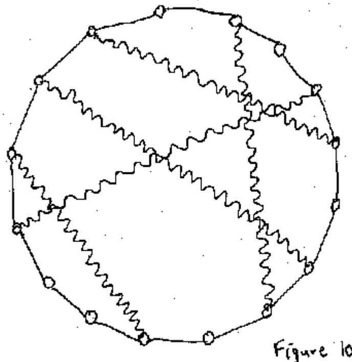
*Figure 10. A minimally-connected set of nodes with only nearest-neighbor links is made into a 'small-world' network by adding a few longer links.*
